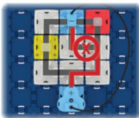
Make sure to avoid creating “short circuits” such as those shown above, where the current can move completely through the circuit without passing through an LED. **Always remove the Power Supply tokens from the grid when Circuit Maze is not in use.**
