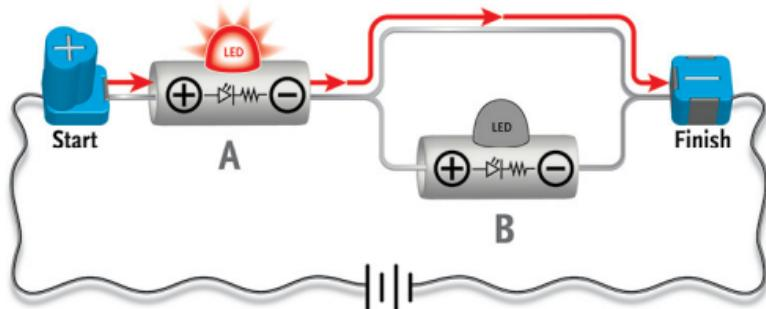
Beacon in parallel with bypass metal strip in series with another Beacon –
