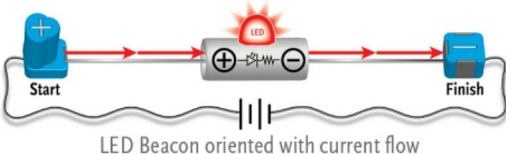
As shown in the following diagram: If the LED Beacon is reversed so that the (-) side faces the Start Token (+), the LED valve closes and current does not flow through the LED. The Beacon stays dark.
